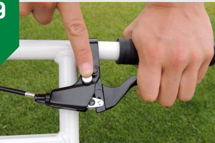
To keep the discs off the ground permanently press the button on the handle while squeezing it.
