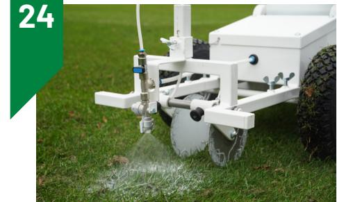
Return ball valve to horizontal position to rinse spray head and nozzle.
