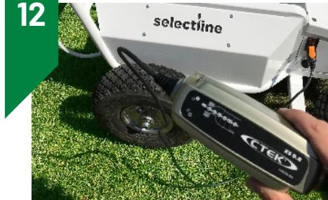
Connect the charging plug to the machine and the charger to a 220V socket. An indicator light tells you the charge level. The battery is fully charged when the '5' lights up green.
