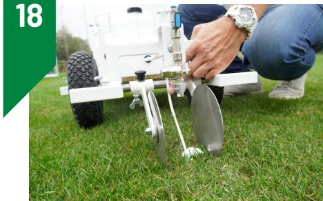
As soon as paint comes out, return the ball valve to horizontal position.
