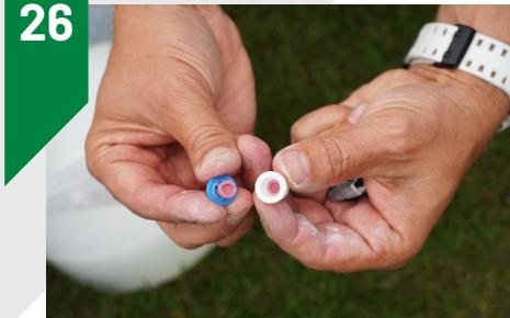
Separate all parts and disassemble the nozzle.
