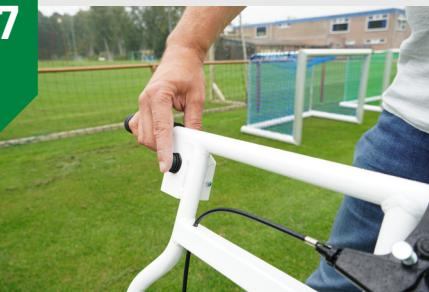
Switch on the machine and rinse until paint comes out.
