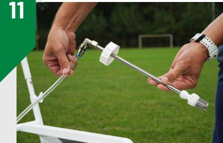
Connect the tube to the suction rod.
