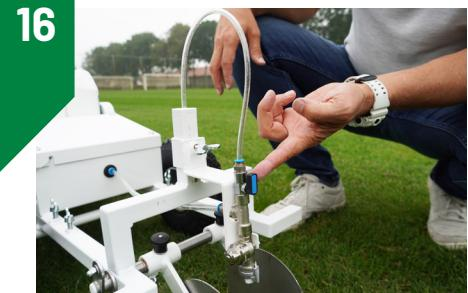
Turn the ball valve to vertical position.
